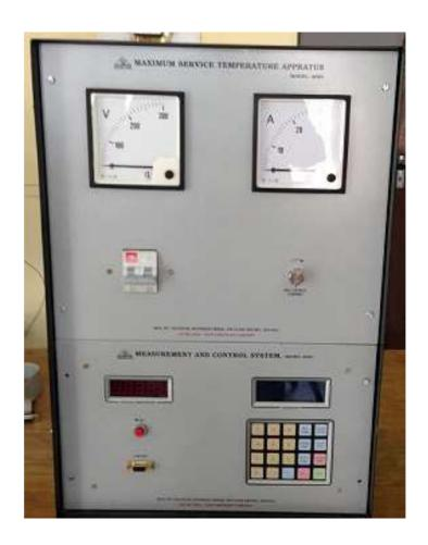
Maximum Service Temperature Apparatus (DG-IS-MSTA), is a microprocessor based instrument designed to measure and display the Thermal Resistance of loose filled insulating materials, using hot plate method as per guidelines of Standard: EN 14706. The instrument is automatic and programmable; designed with latest integrated circuit technology. The instrument displays the measured value directly in engineering units.
