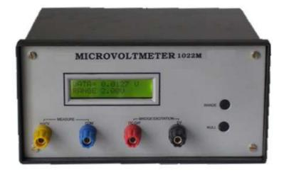
The **Digital Micro Voltmeter (DG-ME-DMV),** offers a wide DC voltage measuring capability at moderate cost. High accuracy and resolution, high reading rate and constant input resistance are assured. It employs dual slope integration technique for analogue to digital conversion. This multi-purpose equipment is useful in general laboratory and R&D labs for the measurement of low DC voltage.
